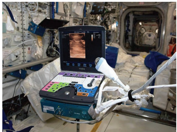
Figure 50-1 The International Space Station (ISS) Ultrasound System (Vivid Q, General Electric, Waukesha, WI) is ready for use. The box underneath the machine is a data and power interface. Note the oversized water drop on the 12-MHz linear array transducer, to be used for acoustic coupling instead of gel. Also note the multicolor keyboard overlay specially designed for remote guidance purposes. (Image courtesy National Aeronautics and Space Administration.)
